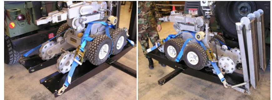
Secure arm with bungee cord (helps reduce damage to arm when transporting).
